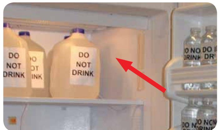
Water bottles in refrigerator to absorb cold air blown in from freezer to reduce risk of vaccines becoming too cold
